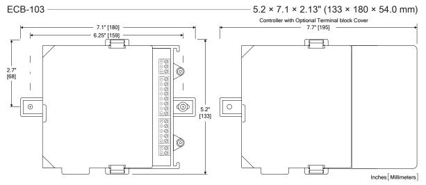
Shipping Weight: ECB-103 0.92lbs (0.42 kg) Enclosure Material<sup>1</sup> FR/ABS Enclosure Rating Plastic housing, UL94-5VB flammability rating Plenum rating per UL1995
